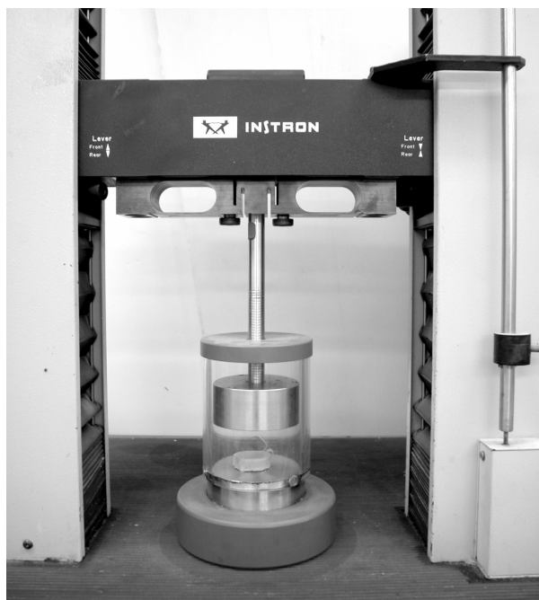
Figure 7. Device used for the compression of cellular solids and for an acoustic recording of their response (courtesy of N. Jaffe).
